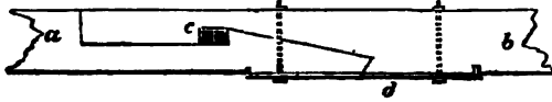
Fig. 89—Represents a scarf joint arranged to resist a cross strain and one of extension. The bottom of the joint is secured by an iron plate confined by bolts. The folding wedge key inserted at c serves to bring all the surfaces of the joints to their bearings.
